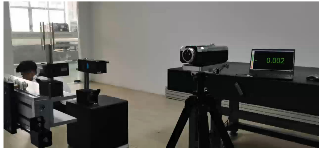
The vibration testing of the measurement module
