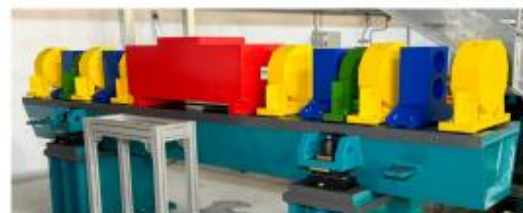
Prototype of the magnetic elements of the new storage ring lattice
