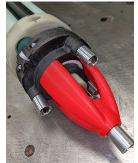
PCB probes stiffened with carbon fiber or G10
