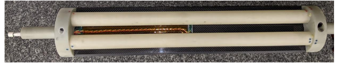
PCB probes stiffened with carbon fiber or G10
