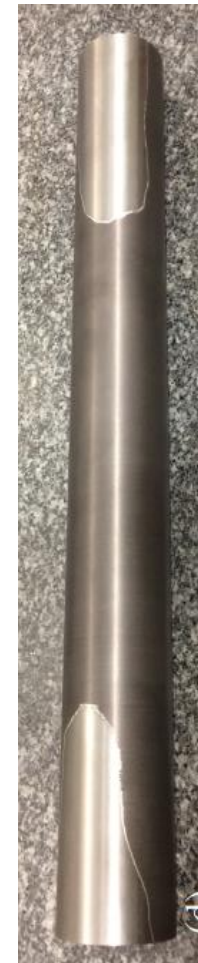
gradual penetration from end flux jumps at lower field on ramp-down
