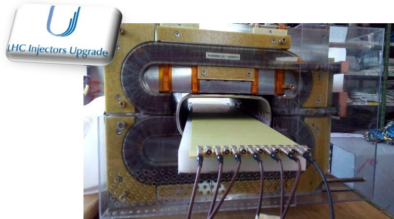
new PS extraction bumper with pole face loops for passive sextupole compensation
