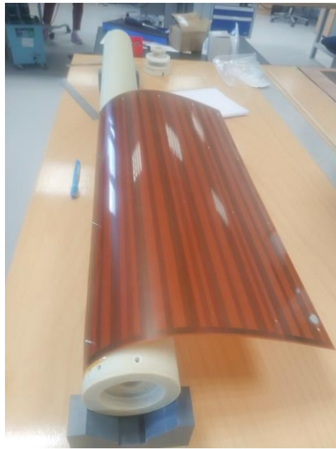
2 x double-layer flexi PCB glued together 4 x 16-turn tangential coils per layer
