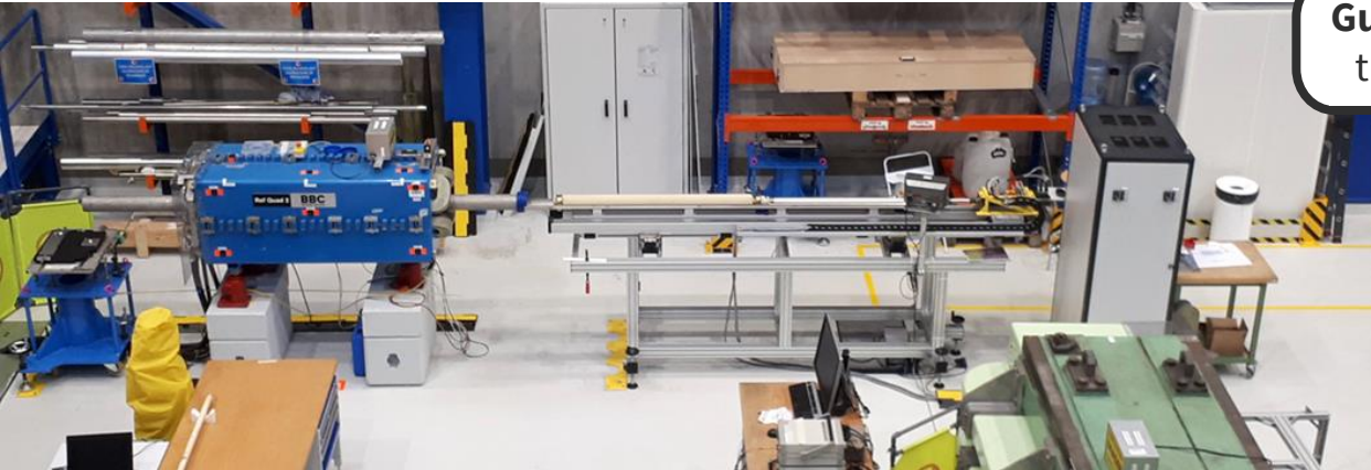
Quadrupole calibration setup based on CERN-standard rotating coil system
