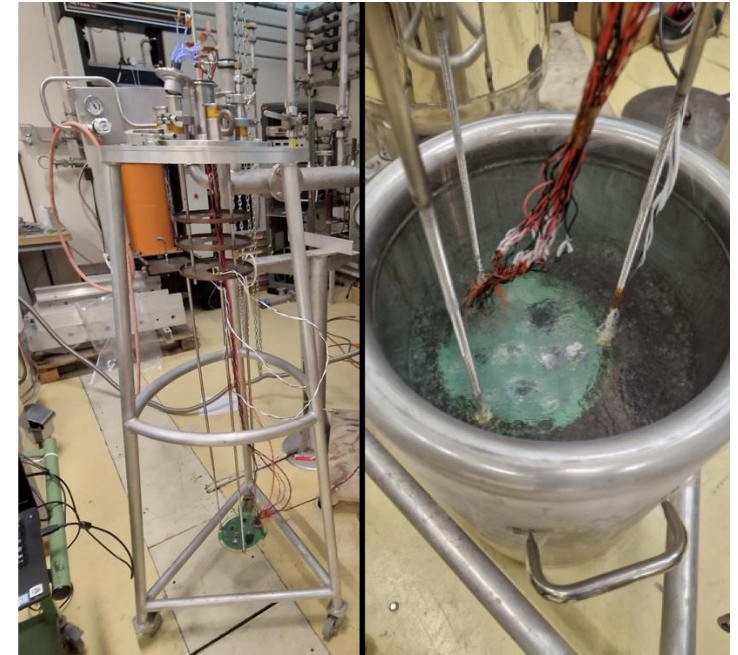
Assembled test head (left), liquid nitrogen tests (right).
