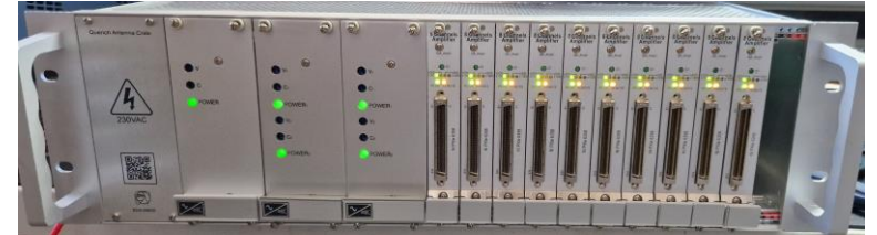
Custom design of amplifier cards and crates for Quench Antenna.
