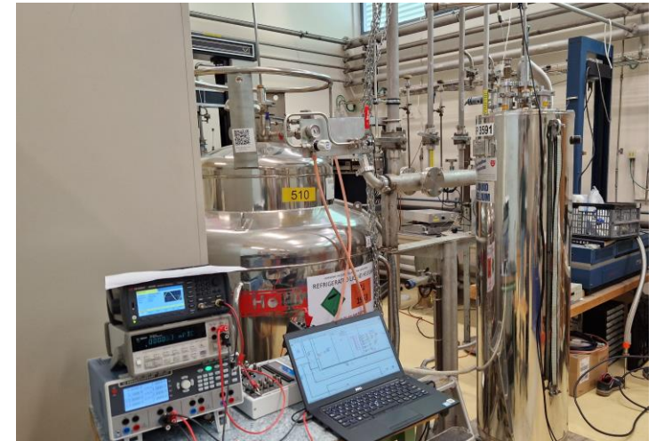
setup for the test in liquid Helium at 1.9 K.
