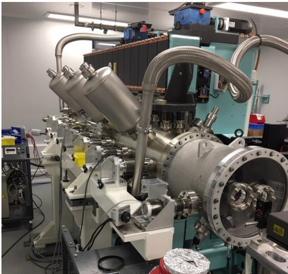
CPMU18 (2017) with the Hall Probe bench inside the vacuum chamber
