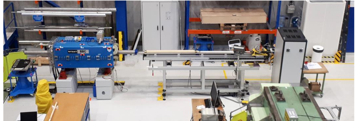
The radii calibration bench in bdg 311 installed on RefQuad2 magnet
