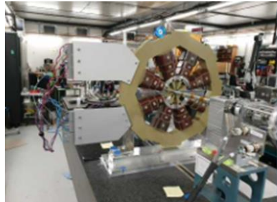
Field Quality and Field Integral tuning with Rotating Coils: Contribution C. Zoller
