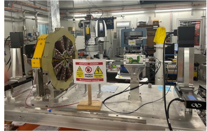
Sextupoles & Octupoles axis measurement with vibrating wires: Contribution M. Aiba
