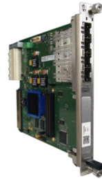
DAMC2 Required for Clock & Control system for fast 2D detectors, VETO System, Machine Protection System and photon beam loss monitors from DESY
