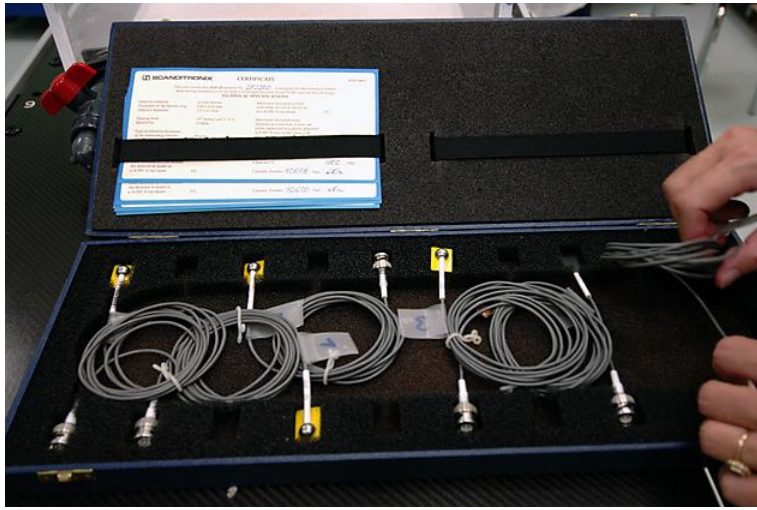
Set of diodes for in-vivo dosimetry
