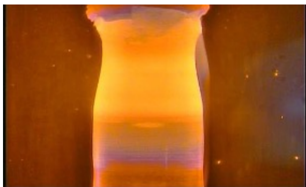
Single crystal growth process of solid state laser material Nd:YAG in laser furnace [1].
