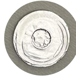
Sealed coin target (In wire) to prevent oxidation during transport, installation, removal
