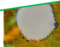
Thickness = 13 \mu\text{m} (50- \mu\text{m} -thick gold substrat) m(Gd): 2-3 mg (ICP-OES analysis)
