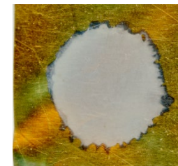
Thickness = 13 \mu\text{m} (50- \mu\text{m} -thick gold substrat) m(\text{Gd}) : 2-3 mg (ICP-OES analysis)
