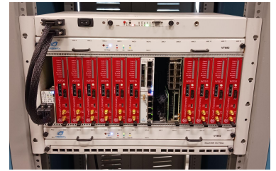
WFD5 crate @ TRIUMF. 10 modules x 5 channels = 50 channels. Will eventually need 1-2 more crates for all PMTs.
