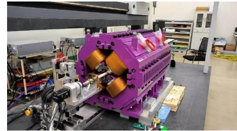
Measuring BD magnet with CMM based Rotating coil system
