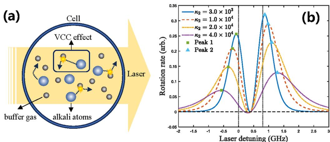
Figure 5: (a) VCC effects in buffer-gas filled vapor cells.(b) Simulations of the rotation rate spectra for different laser power
