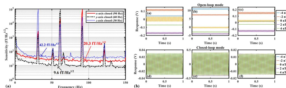
Figure 9: Results of triaxial dynamic measurement. (a) The triaxial measurement sensitivities of an OPM in the closed-loop mode. (b) Measurements of sinusoidal calibration signals under residual magnetic field fluctuations.
