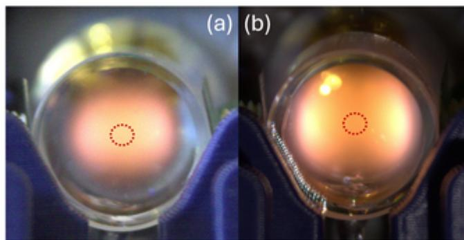
Figure 4: Helium plasma in the glass cell for (a) weak and (b) high plasma supply voltage
