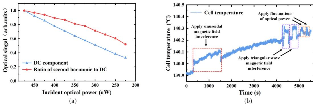
Figure 7: (a) The variations of the second harmonic to DC ratio and the DC component itself with the incident light power. (b) Long-term evaluation of thermal control performance under external disturbances.
