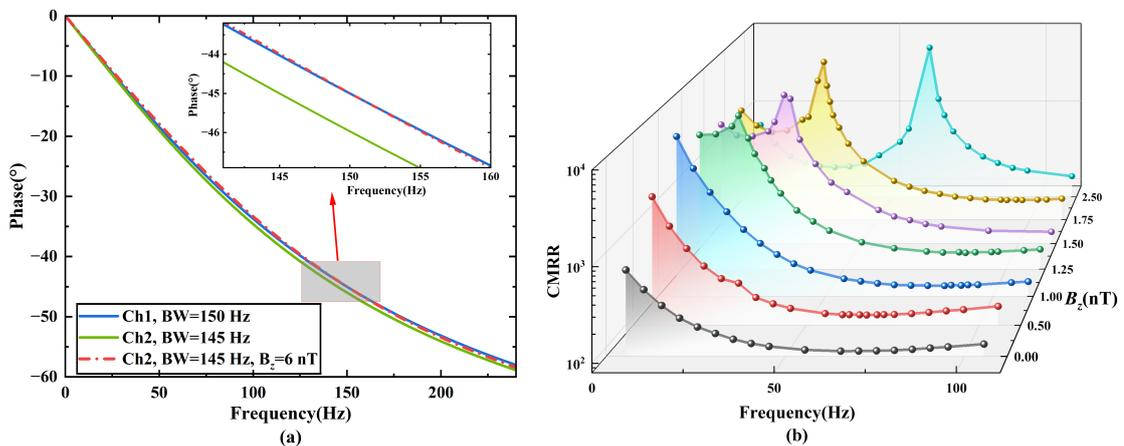
Figure 6: (a) Simulated phase-frequency response of OPMs with different bandwidths. (b) Variation of CMRR with signal frequency under different  $B_z$ .
