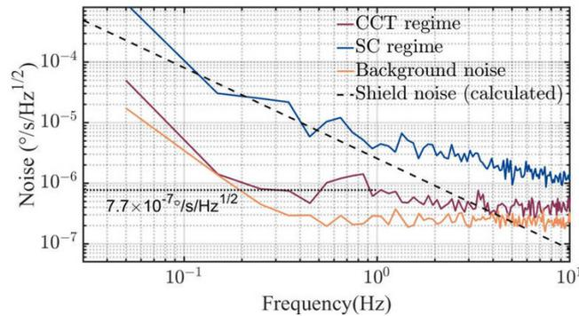
Figure 2: Noise spectrum of the comagnetometer. The background noise is obtained from the noise spectrum of unpolarized atoms. The shield noise, arising from the ferrite magnetic noise, is calculated based on the measured data.
