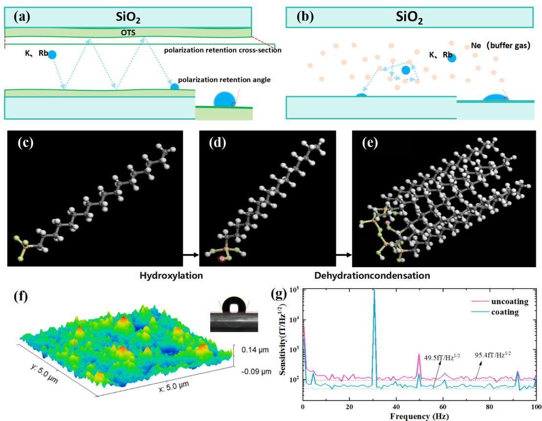
Figure 8: (a) Relaxation of coating cell, (b) relaxation of uncoating buffer gas cell, the molecular cross linking process of OTS : hydroxylation(c to d) and dehydration condensation(d to e), (f) AFM and contact angle test of OTS SAMs, (g) sensitivity of coating and uncoating magnetometer
