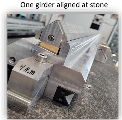
Magnetic tuning of single girder with Hall probe
