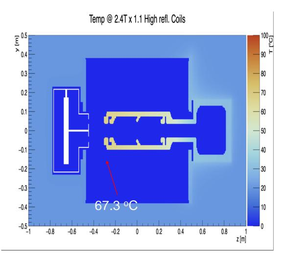
Passive heat flow simulations show that heat will not conduct quickly enough out of the chamber via the support structure. Active cooling will be needed.
