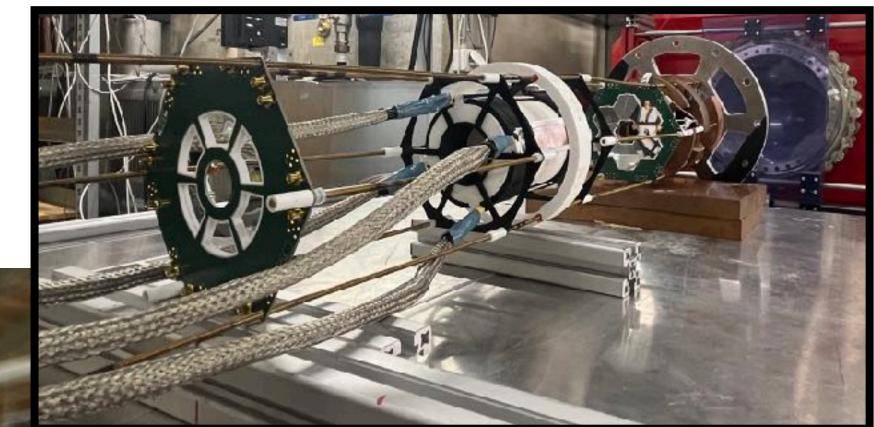
Sept beamtime established that a grounded braid around each of the coaxial cables significantly shields the detectors from the kicker pulse.
