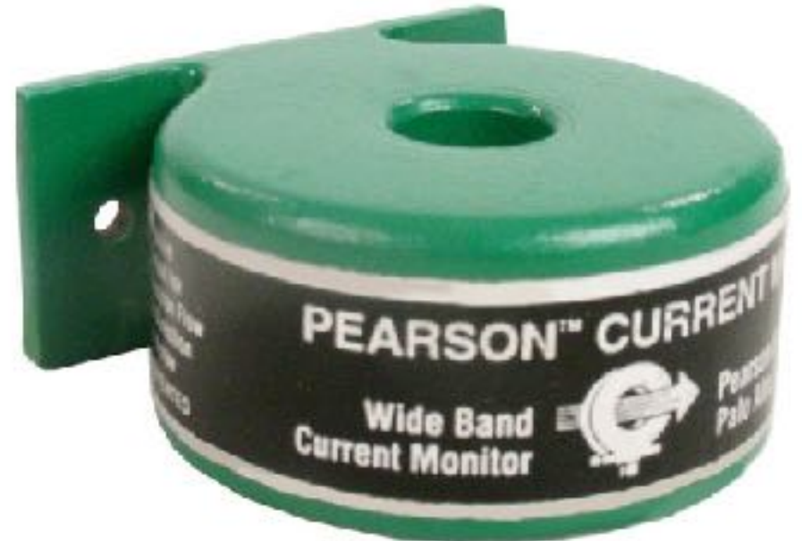
Current measured using Pearson wideband current monitor with -3dB at 20MHz and 0.1V/A output
