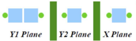
FIG. 28. Scintillating fibers and WLS fiber arrangement.
