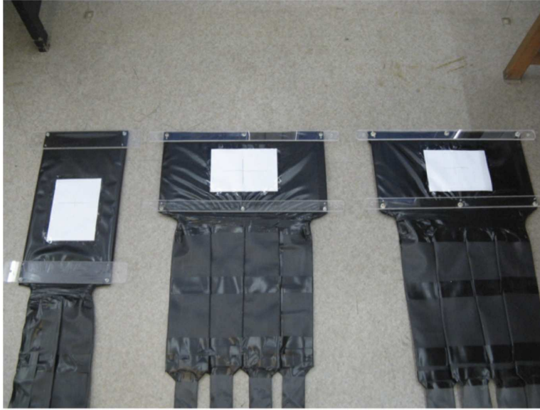
FIG. 27. 3 SciFi planes to be installed for the test beam, one plane in the IFP and two near the target.
