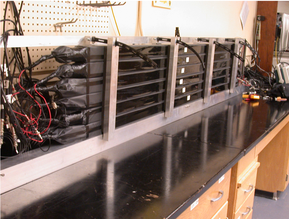
Scintillation bars for the CLAS12 FTOF detector under cosmic ray tests at USC
