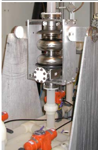
BCP cavity etch
