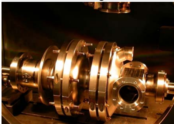
E-beam welding of cavities
