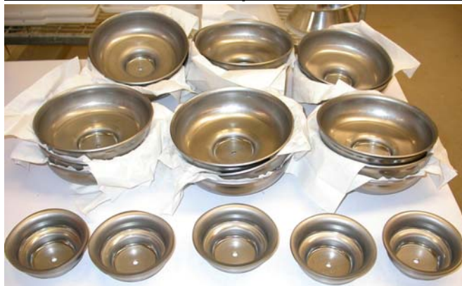
Pressed Nb cups for cavities
