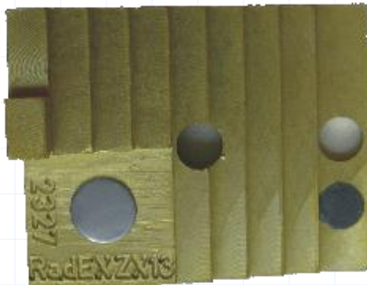
Calibration sample – Aluminum made steps with thickness from 1.8 mm to 15 mm
