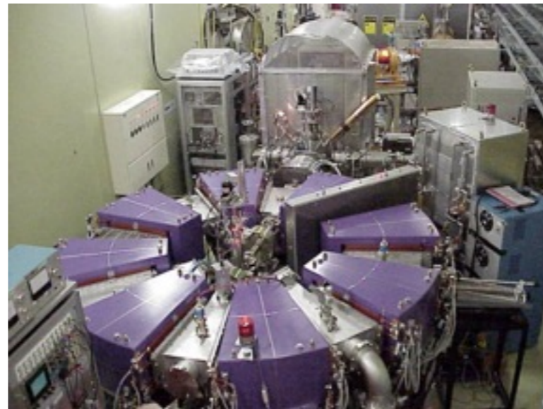
PoP 1 MeV proton FFAG with 1 kHz operation in 1999
