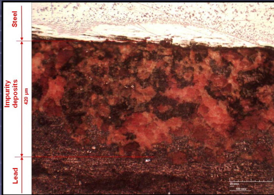
Picture of Sample Wall Boundary Area ( T= 550^{\circ}\text{C} , t=100 hours, a=10^{-1}-10^0 , Q=0.55 m 3 /h, V=2 m/s, Re=1.074*10^5 ) at 200-Fold Magnification
