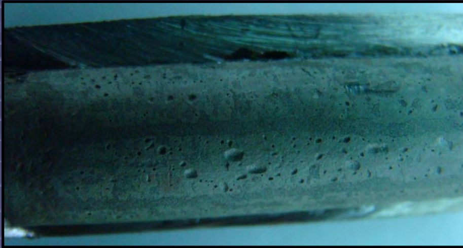
Gaseous (Gas-Vapor) Cavity in Lead Ingot ( T= 450^{\circ}\text{C} , t=22 hours, a=10^{-2} , Q=0.27 m 3 /h, V=1\text{m/s} , \text{Re}= 5,394*10^4 )
