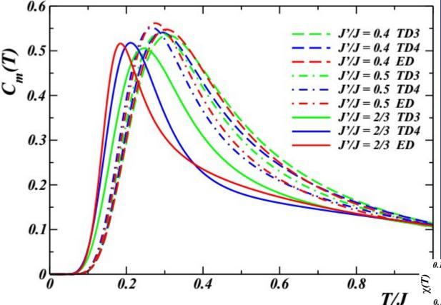
Even-length clusters contain low-lying singlets close to the gap energy and provide a more accurate account of the magnetic specific heat. However, for coupling ratios near the QCP they fail to reproduce the anomalously low peak position.
