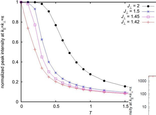
The spectral weight remaining in one-triplet band for the fully frustrated ladder falls with increasing T; this decrease is very abrupt near the QCP due to the proliferation of manytriplet bound states.
