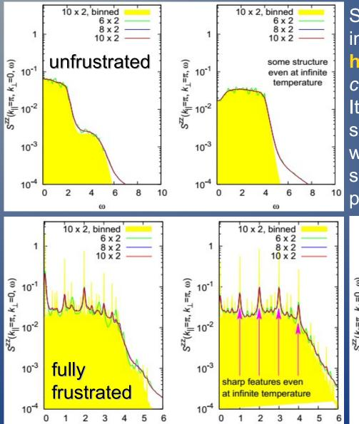
Sharp spectral features remain present in the fully frustrated system **at the highest temperatures**. *This is a consequence of the discrete support.* It contrasts strongly with the flat spectrum of the unfrustrated ladder, which shows only separate triplet sectors. Nearly-flat bands give finite peak widths at infinite temperature.
