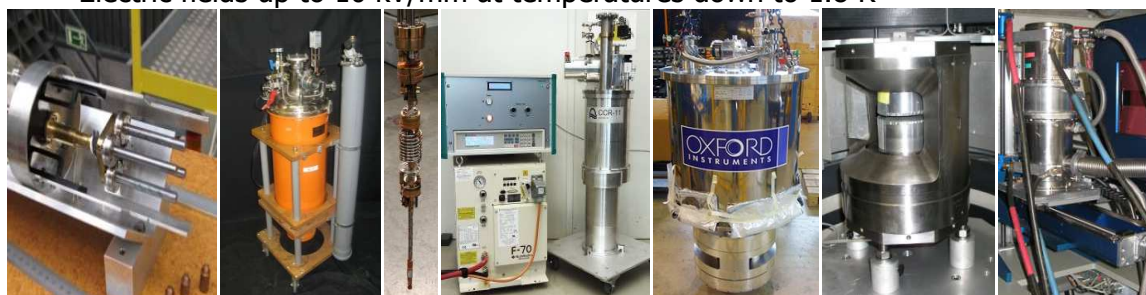
Figure 16 From left to right: multi low temperature sample changer, orange cryostate, closed cycle cryostate, cryomagnet, pressure cell, high temperature furnace. (Pictures PSI, ILL, FRM2).
