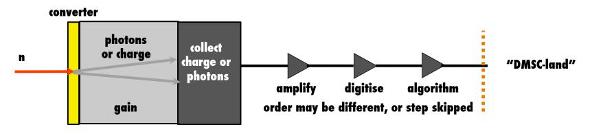
"Converter" "Detector" "Electronics"
