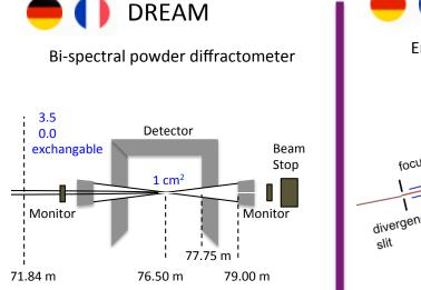
PD detector size: ~9.7 m<sup>2</sup> (6.2 sr). Pixel size: 4 mm x 4 mm.
