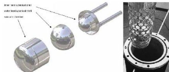
Figure 4.2. Left: The core of a new cold moderator design, a hemispherical container for the moderator liquid H_2 . [Knop and Schreiner, Geesthacht, 2010]. Right: The present moderator at JEEP II.
