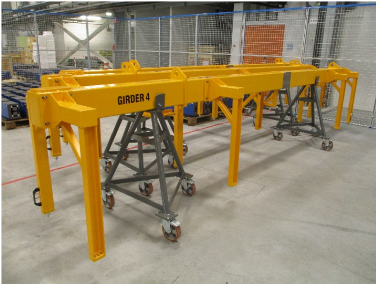
vacuum chambers assembly handling tool
