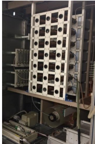
Pulse forming network 525 nF, 21.5 mH
