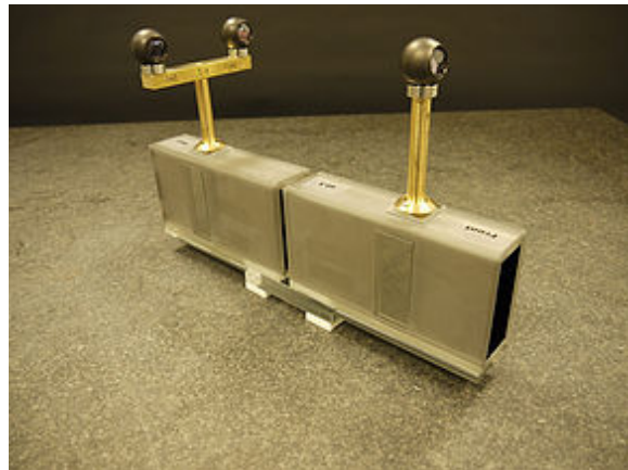
The extensions have three ceramic spheres, which fits perfectly to the alignment plates. The repeatable accuracy is 5 microns.
