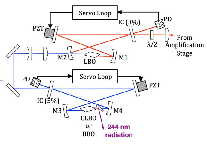
Upgrade laser system used for positronium
