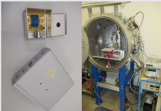
Si-sensor and DAQ system (left) Monochromator chamber (right)
