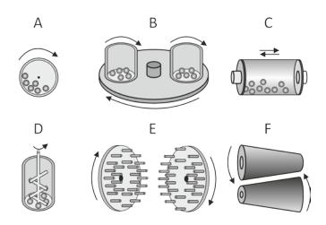
Types of mills for high-energy milling: A: ball mill, B: planetary mill, C: vibration mill, D: attritor (stirring ball mill), E: pin mill, F: rolling mill.
