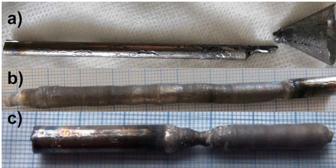
FIG. 1: Photos of a) the cast \text{CeAlGe} rod, and the floating zone grown crystals of b) \text{CeAlGe} and c) \text{PrAlGe} .
