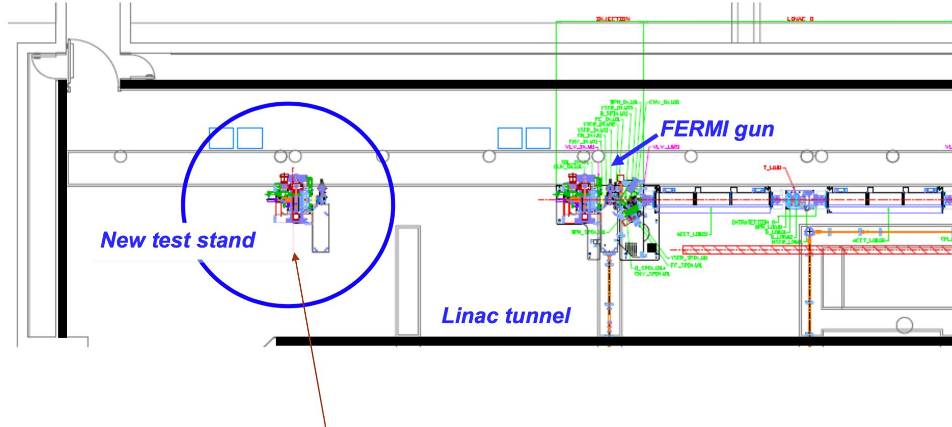
Layout of FERMI linac tunnel. The CTF has been installed in a free space behind the FERMI photoinjector.
