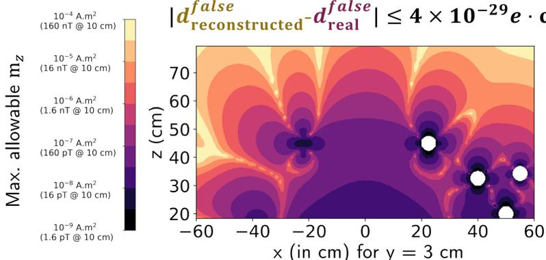
Such a map of the whole volume gives the limit of the allowable dipole strengths  $m_z$ , below which their effect on the CsM array's performance is negligible.
