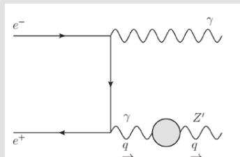
Looking for a single monochromatic photon with missing energy
