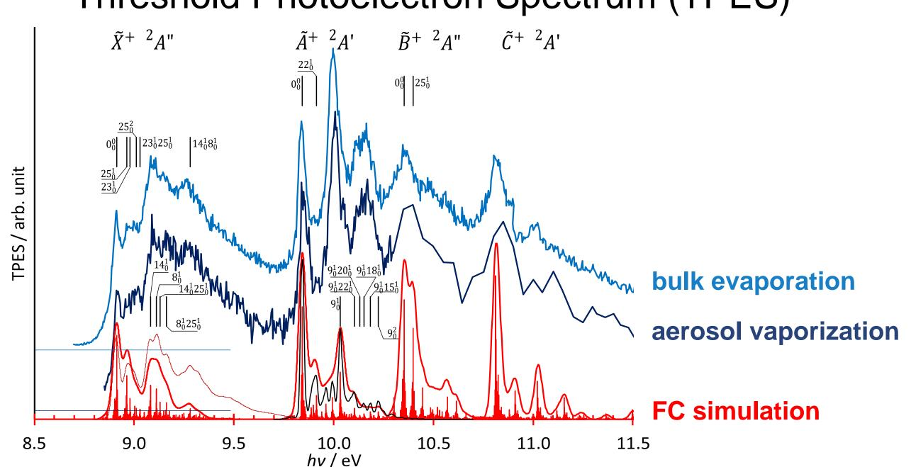
Franck-Condon factors (FCFs) for vibrational transitions are convoluted with a Gaussian to account for thermal broadening.
