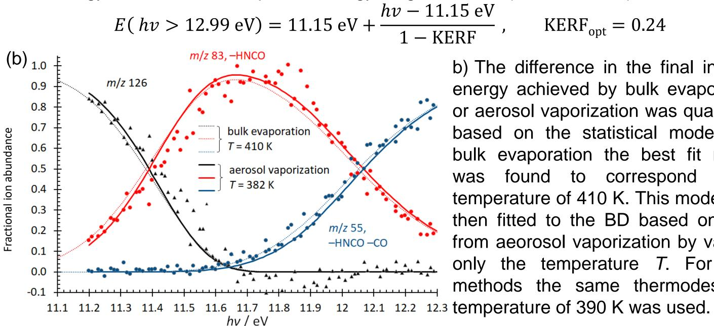
b) The difference in the final internal energy achieved by bulk evaporation or aerosol vaporization was quantized based on the statistical model: For bulk evaporation the best fit model was found to correspond to a temperature of 410 K. This model was then fitted to the BD based on data from aeorosol vaporization by varying only the temperature T. For both methods the same thermodesorber
