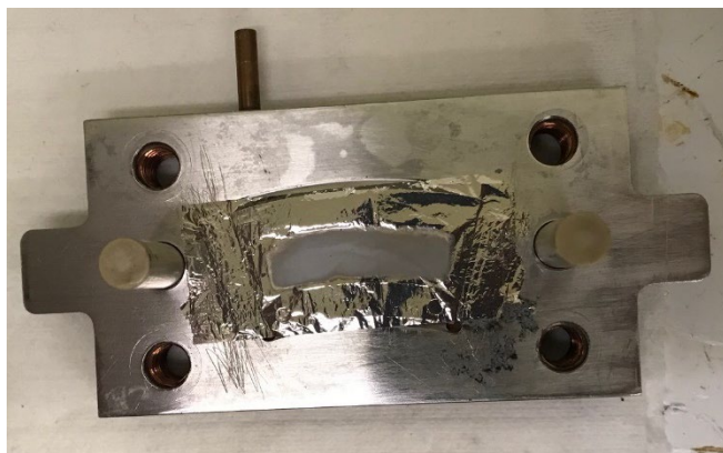
1. Deposition unit disassembled
