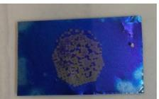
395 µg/cm<sup>2</sup> Th-232 on 25 µm Ti foil
