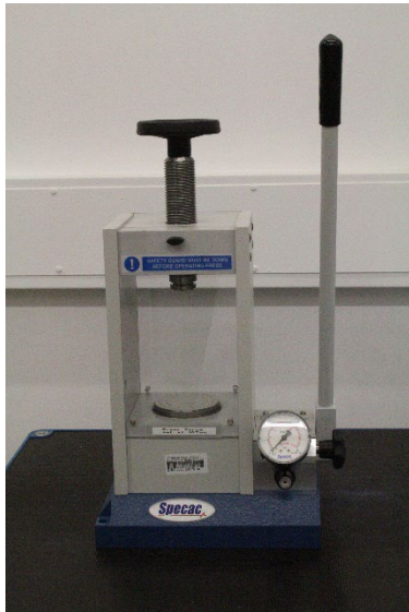
Specac press 15-t pressure load
