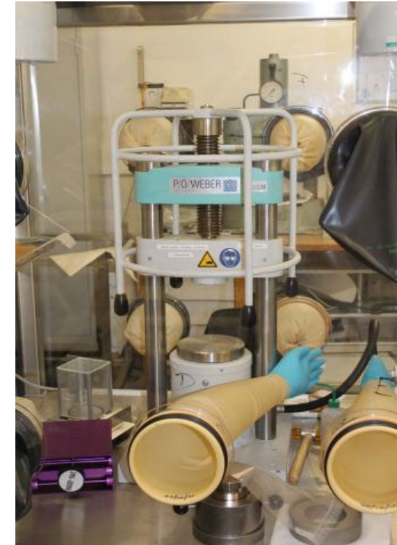
P/O/Weber manual press, Model PW 30-BOX, enclosed in a glove box
