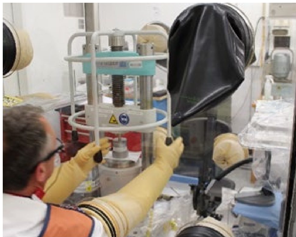
André Moens turning the spindle down of the P/O/Weber manual 2-Column Laboratory Press, Model PW 30-BOX in a glove box and outside the glove box pumping the oil to raise the piston and reaching the designated press force shown on the gauge.
