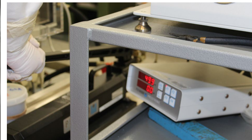
André Moens turning the spindle down of the P/O/Weber manual 2-Column Laboratory Press, Model PW 30-BOX in a glove box and outside the glove box pumping the oil to raise the piston and reaching the designated press force shown on the gauge.
