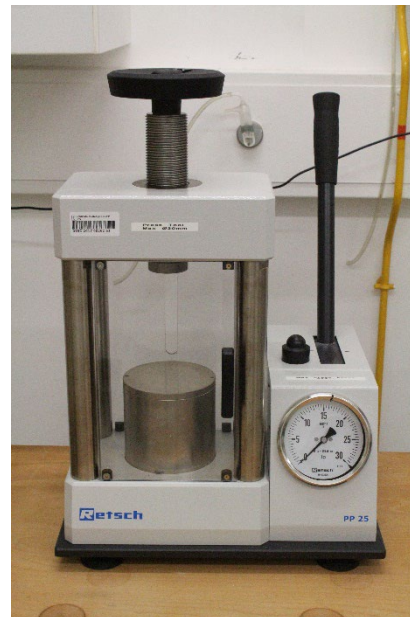
Retsch press 25-t pressure load
