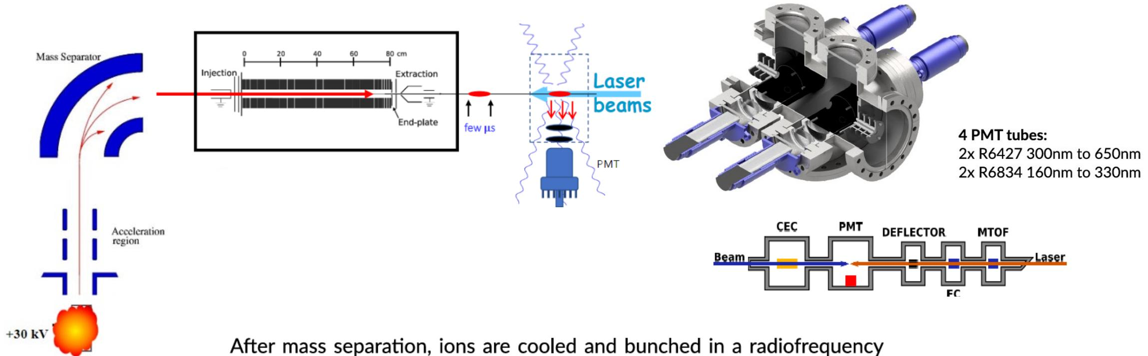
After mass separation, ions are cooled and bunched in a radiofrequency cooler-buncher, before being reaccelerated to 30 keV and delivered to the collinear beamline. There, ions are overlapped in a counter-propagating geometry with a CW laser beam which excites them from either the ground state or low-lying metastable state. Detection of laser-induced fluorescence allows the measurement of IS and HFS from the frequency pattern
