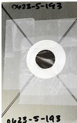
\text{Cs}_2\text{IrCl}_6 precipitate on filter for counting 11mm diameter
