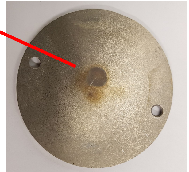
Niobium disc used as energy degrader
