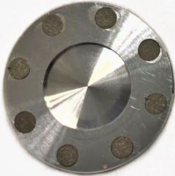
Covering lid: degradation of the impinging energy to the desired value
