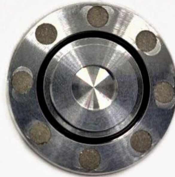
Containing cup: complete stopping of the proton beam
