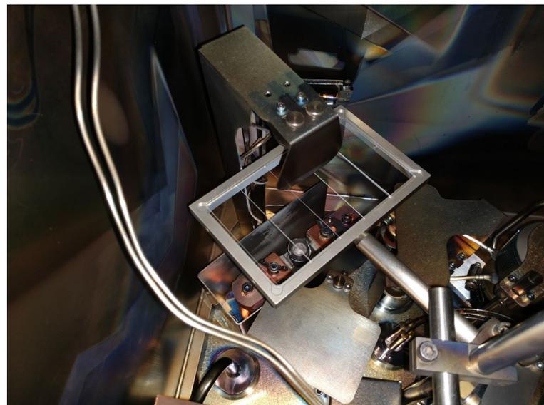
Set-up for substrate evaporation of NaCl
