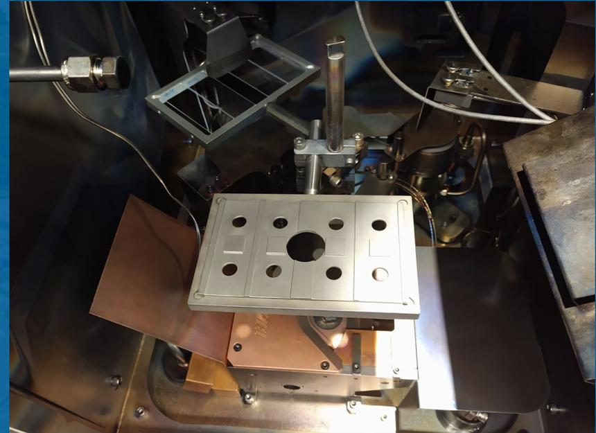
Deposition set-up for the NaCl substrates (rear) and carbon backing foils (front)
