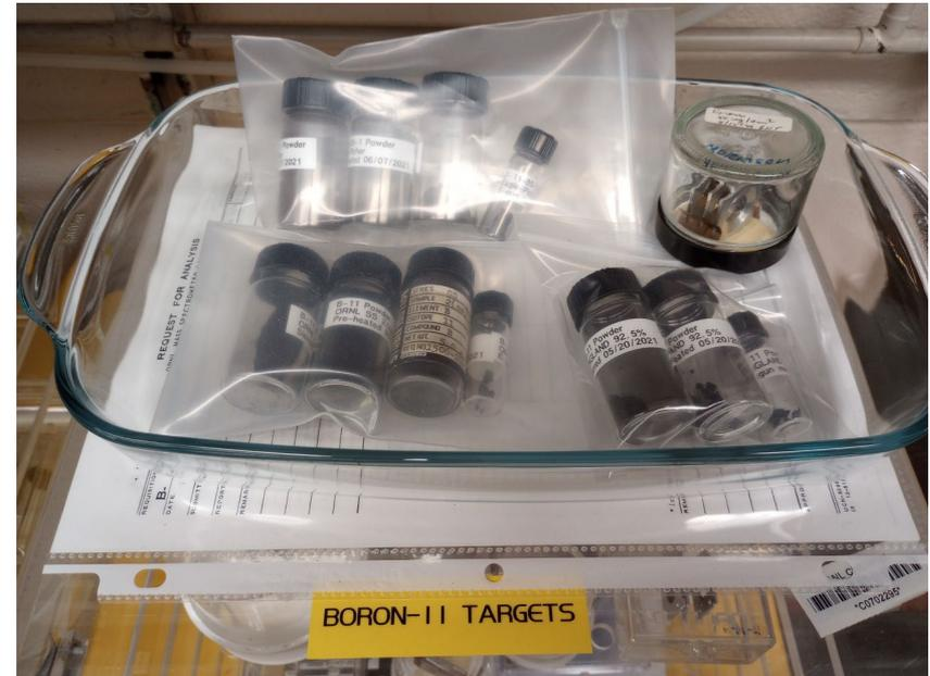
Collections of various milled, sieved and ,melted isotopic boron samples
