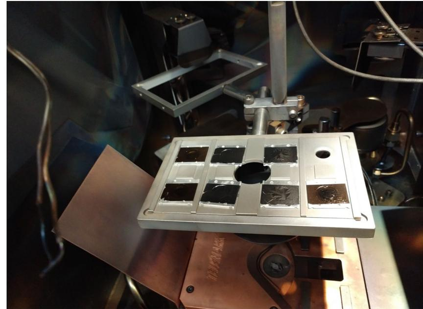
Angstrom Deposition Tool set-up for evaporating boron onto carbon backings
