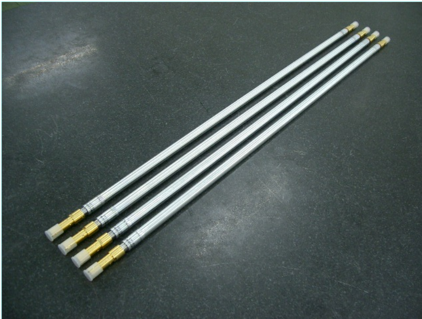
Position sensitive neutron detector Made by Aluminum Alloy
